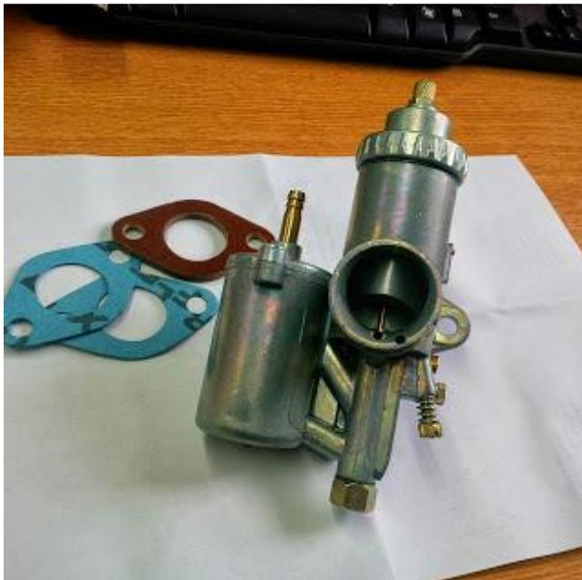
The flange holes were too close together to fit on the cylinder head spigots. Cured with an 11 mm drill and round file. Tests with fuel on led to fuel pouring out of a tiny bleed hole on the float chamber cover joint. Tests of same thing with original carb did the same thing. The carb supplier sent over a complete new aftermarket carb this time with hole blanked off. No more leaks plus I now had 2 identical new carbs plus the old one. Bike still ran rich though.
