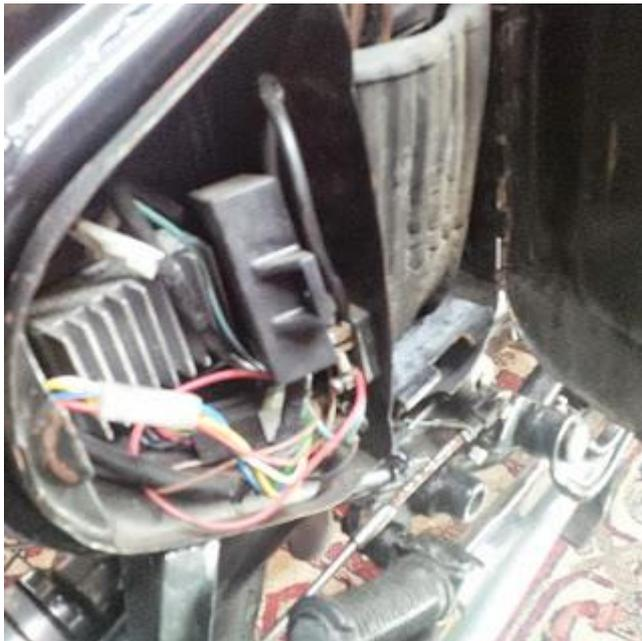
Battery box wiring tidied up and secured + trickle charger socket wired in
