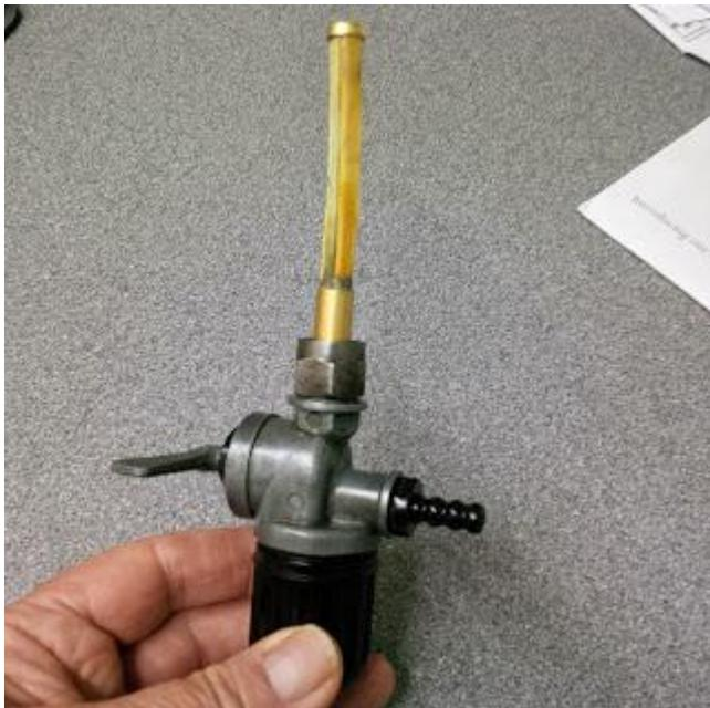
Replacement refurbished original fuel tap with horizontal outlet
