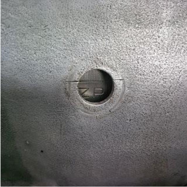
This peep hole reveals 2 stamped settings as flywheel is rotated. Here is ZP Zundepunkt – 10 degrees before further rotation reveals OTP Oberen Tot Punkt - TDC
